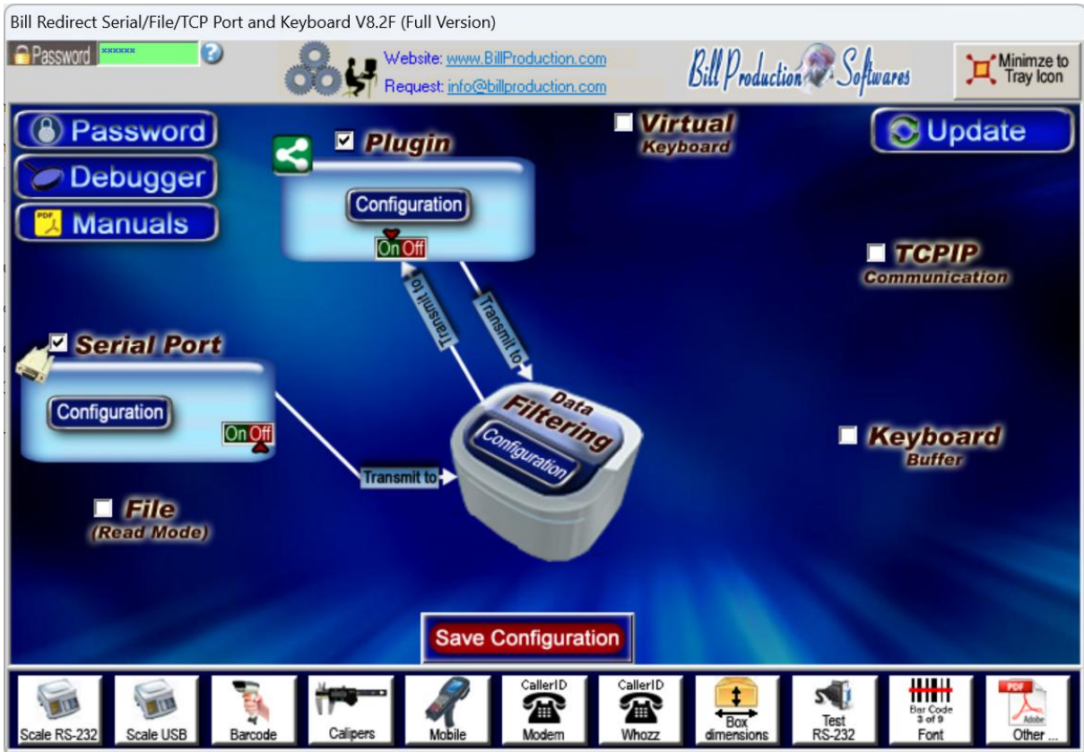
Screenshot: a RS-232 device (Serial Port ON) redirected through Data Filtering to the Plugin (ON).
