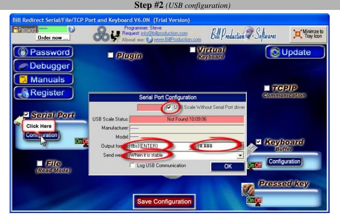
Activate the option: USB Scale Without Serial Port driver
