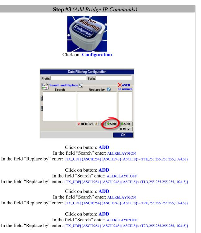
\* To control the relay of a specific Bridge IP replace 255.255.255.255 by the Bridge IP address.
