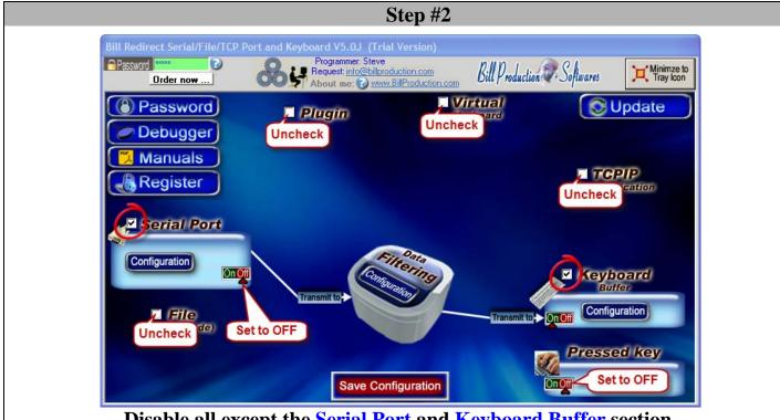
Disable all except the Serial Port and Keyboard Buffer section. Set to OFF Serial Port and Pressed key switch.
