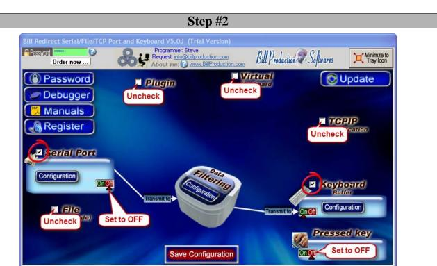
Disable all except the Serial Port and Keyboard Buffer section. Set to OFF Serial Port and Pressed key switch.
